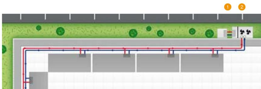
The **1** backcooler and the **2** pump station form the compact and highly efficient waste heat system.
