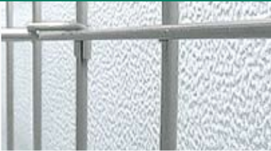
1.) Inner wall prior to the autodefrost process beginning
